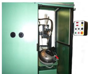
Circular automatic device KMO 111 with rotary table WP 200 is designed for welding the flange. The movement of torch is pneumatic. The control system has program for welding  $360^{\circ}$  plus over beginning of weld.
