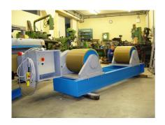
Each unit is constructed from basic frame, wheels' carriers, wheels and supporting carrier in case of movable version. Rim of rotating ball-bearing wheels is hard-rubber
