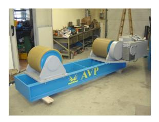
Roller beds-load capacity 100 T, with dust protection.
